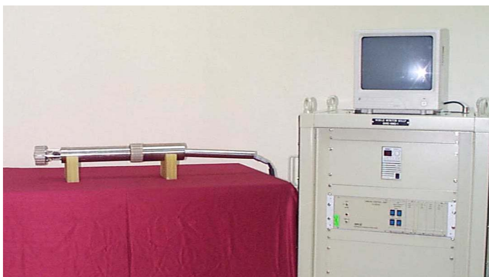
Fig. 1 - Miniature Underwater Radiation Resistant CCTV Camera System
